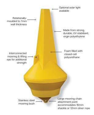
The SL-B700 is extremely long-lasting, and is moulded in strong, durable, UV-stabilised polyethylene. A large mooring chain attachment point accommodates a 16mm shackle or 12mm silver rope.
