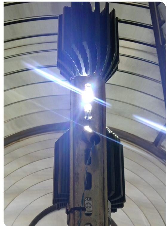
LED Light Source originally developed by the GLA R&R NAV Directorate and manufactured under license to Trinity House.
