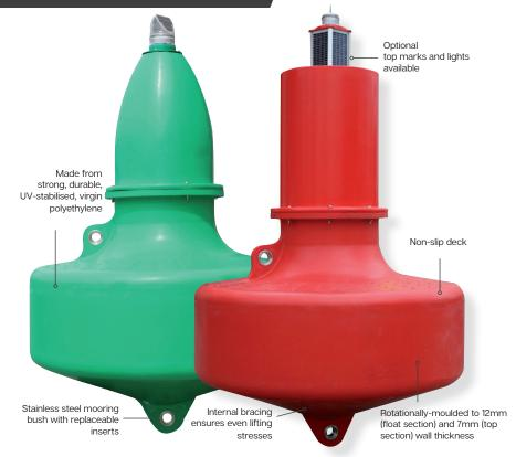
Sealite's SL-B1500 is an extremely robust, high visibility 1500mm diameter navigation buoy perfect for a variety of installations including inland waterways, harbour and coastal navaids.
