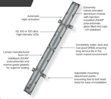
The SL-96 body is made from extruded aluminium with injection-moulded UV-stabilised LEXAN® polycarbonate glass-filled end caps for superior strength and durability. Single, dual and triple row versions have the same body width.
