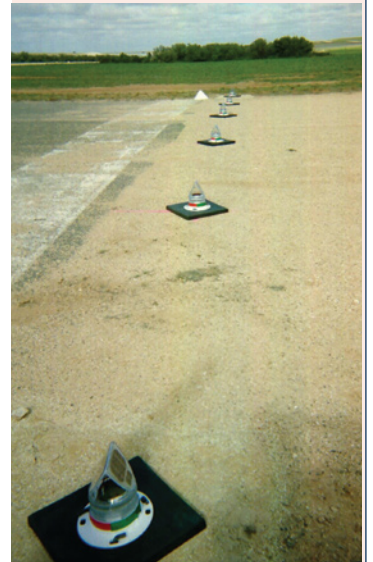
Solar powered temporary airstrip lighting, Loxton Council Airport, South Australia
